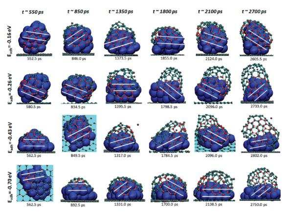
Figure 7. Snapshots showing the correlation between the (110) direction in the Ni<sub>32</sub> nanoparticle and the orientation of the nascent nanotube graphene network at different simulation times.
