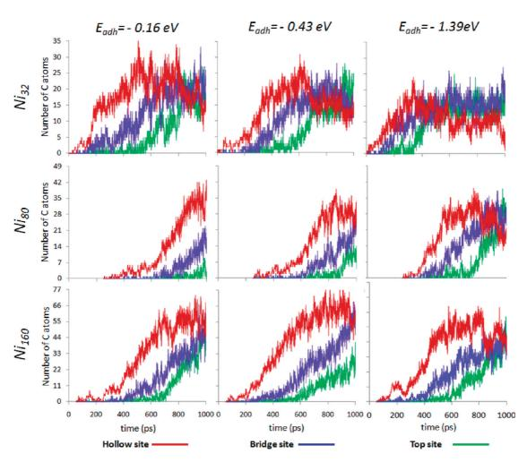
Figure 6. Plots showing the number of carbon atoms occupying each type of site on the nanoparticle vs time.
