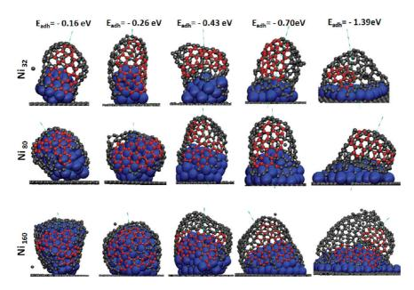
Figure 1. Snapshots after 5.00 ns of simulated growth showing the nascent nanotube structure (red and gray atoms) on supported metallic nanoparticle (blue atoms). The metal/substrate interaction strength increases from left to right, while the nanoparticle size increases from top to bottom; the annealing time before growth was 0.10 ns. Carbon atoms used in assessing the chiral angle appear in red. Green dash-dotted lines are used to indicate the axial direction.
