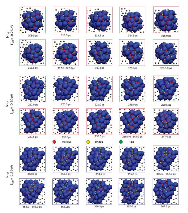
Figure 5. Simulation frames showing the initial formation of ring structures on a supported Ni<sub>32</sub> nanoparticle for three different metal/substrate interactions:  $E_{adh} = -0.26 \text{ eV}$  (top),  $E_{adh} = -0.70 \text{ eV}$  (middle), and  $E_{adh} = -1.39 \text{ eV}$  (bottom). The relevant carbon atoms are colored according to the type of site they occupy on the nanoparticle surface: hollow (red), bridge (yellow), or top (green).
